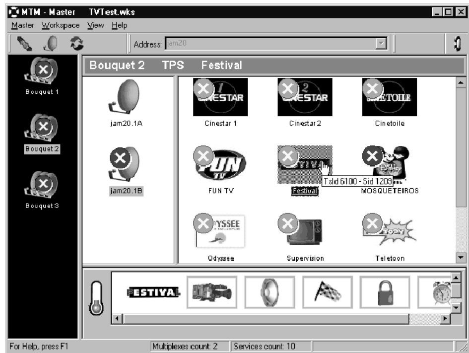
Figure 2- 11: Master client showing errors on a service
